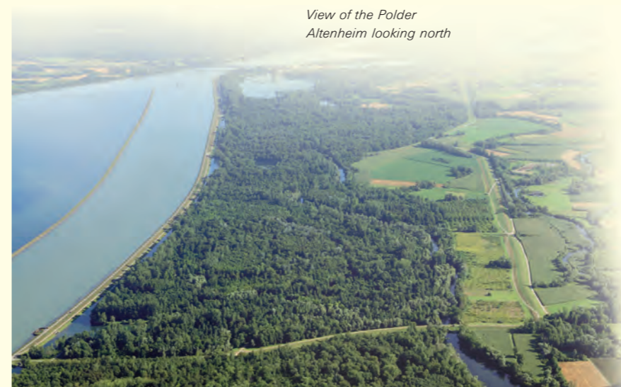
In order to attain the same level of flood protection that existed prior to the systematic development of the Upper Rhine (until 1977), the flood peaks at the Maxau gauging station must be reduced by 700 m³/s, which can be achieved with the IRP retention measures.
